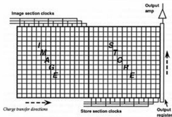
Figure 1. General layout of a frame transfer CCD
